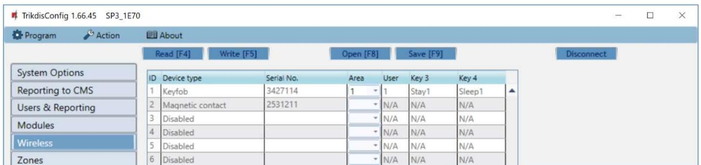
The „FLEXi“ SP3 is compatible with Crow wireless FW2 and Shepherd series sensors, sirens, wireless controllers using the **RF-SH** module.
