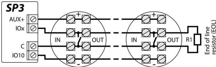
Schematic for connecting two-wire smoke detectors.
