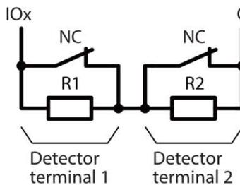
Normally closed with EOL, with tamper and wire fault recognition (ATZ\_T)
