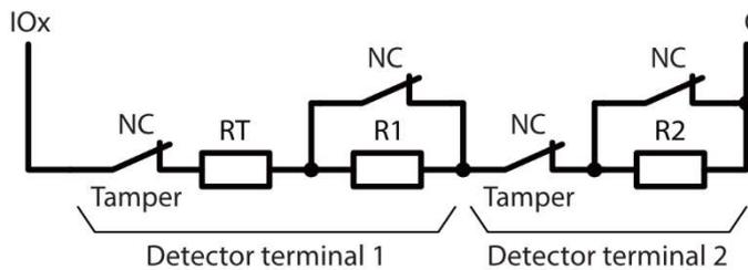
Normally closed with End of line resistor, with tamper and wire fault recognition (3EOL)
