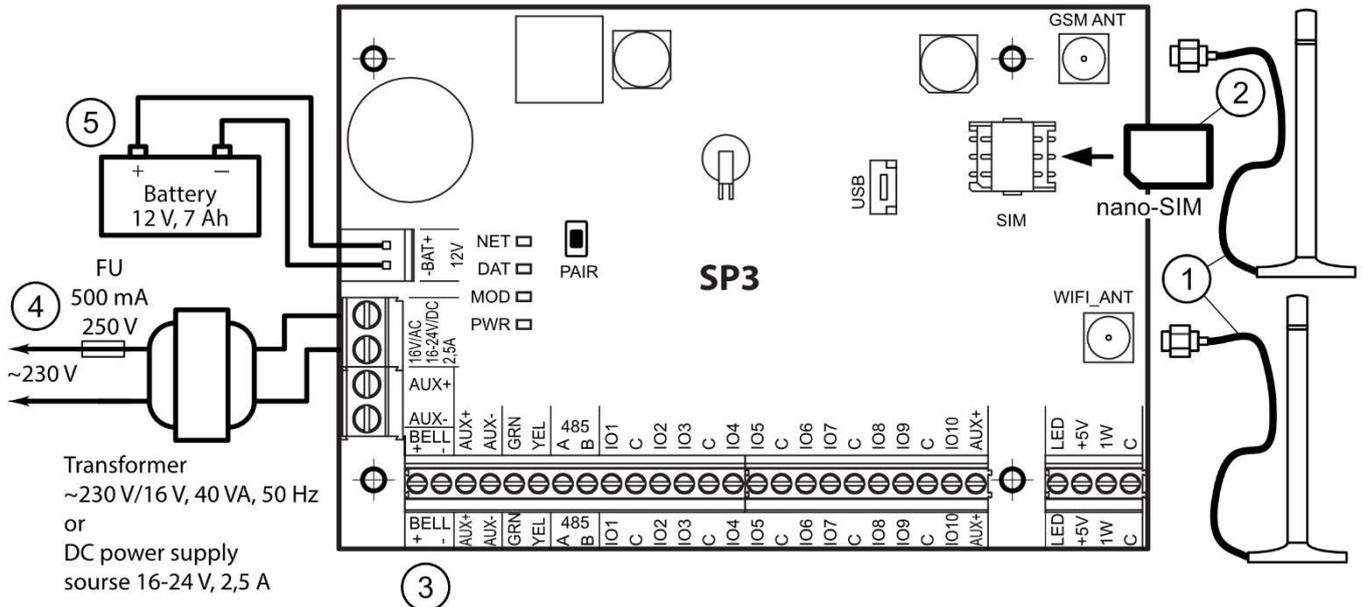
1. Connect GSM and WiFi antennas to the antenna connectors.
