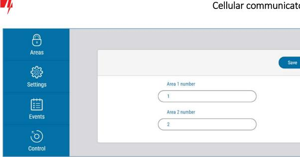
3. In the side menu press Settings and in the newly opened window press Settings. Select the box Arm/Disarm with PGM and specify which area the output will control. One PGM output can control only one area.
