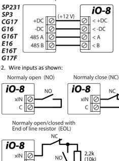
The input wiring diagrams and resistor values are determined by the main unit (*SP231, SP3, CG17, G16, G16T, E16, E16T, G17F*) to which the *iO-8* module is connected.
