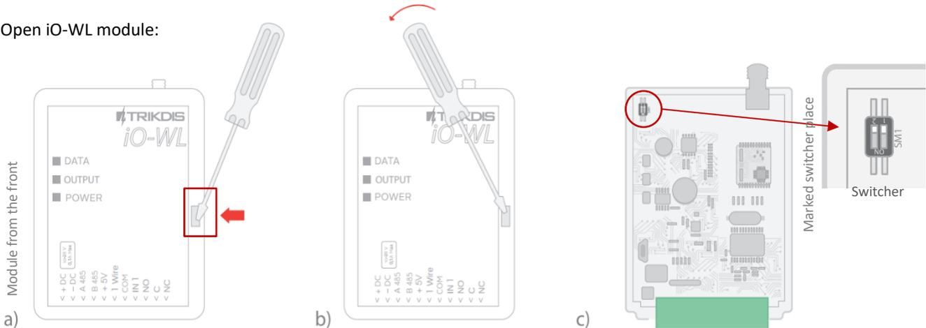
Use **flat screwdriver** to take of front cover. Put screwdriver's head to the marked slot. Hold bottom casing part tightly!
