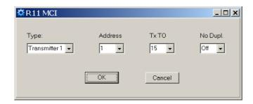
Sending delay Tx TO is applied for sent signal delaying in the radio system. Numerical value repeatable 250 ms.
