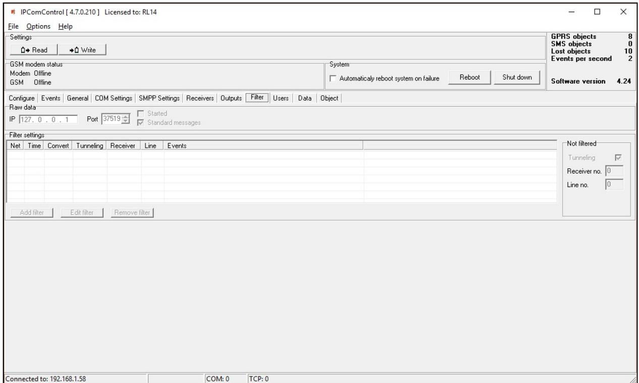
IP address and port number to which all received messages will be sent are entered in field *Raw data*. Messages will be sent to the specified IP address without processing when box [Started] is ticked. Messages will be changed according to protocol Contact ID if box [Standard messages] is ticked.
