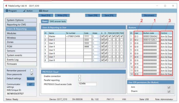
4. When the configuration is done, press **Write[F5]** and all the settings will be stored in the memory of the security panel.
