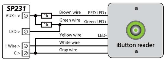
The output LED must be set to the "System State" type. Security alarm is on - the iButton reader light is red. The security alarm is off - the iButton reader light is yellow.
