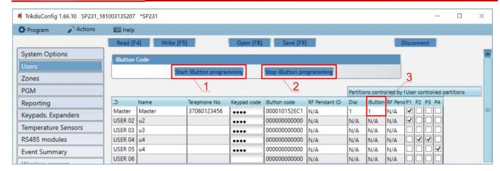
Pairing the IDs of the keys of iButton is performed in the field iButton code:
