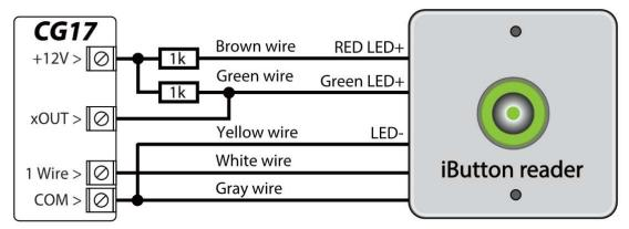
The output xOUT must be set to the "System State" type. Security alarm is on - the iButton reader light is red.
