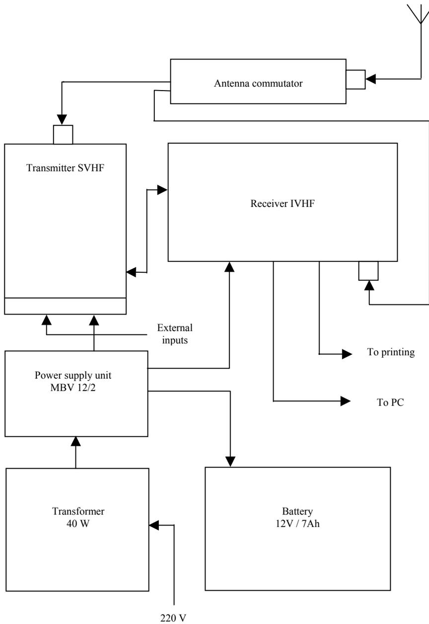
Exploitation parameters and functions of the receiver are set during the configuration of the repeater. These parameters are set: encoding system, time of insensibility to the same message, retransmission mode and format of data output to PC or printer.
