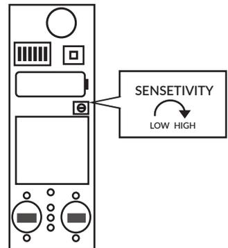
**Preparing the Anti-masking channel for operation (Study Procedure)** (Obligatory for proper anti-masking operation!!!) To enable proper operation of the masking detection (anti-masking), it is necessary to allow the detector to automatically study and analyze the environmental conditions of its protected area. This is an obligatory action that should be performed by the installer, to ensure proper operation of the anti-masking channel!!!
